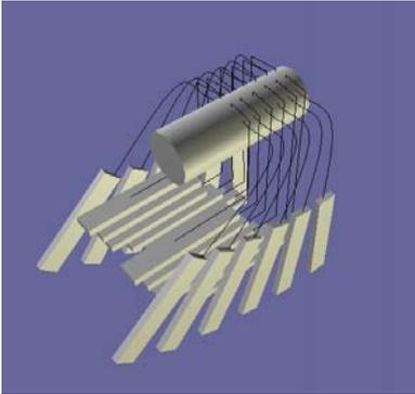
Fig. 4 –Schematic diagram of the tactile array. The finger is represented by the cylindrical element. The mechanism is at the back of the finger.
