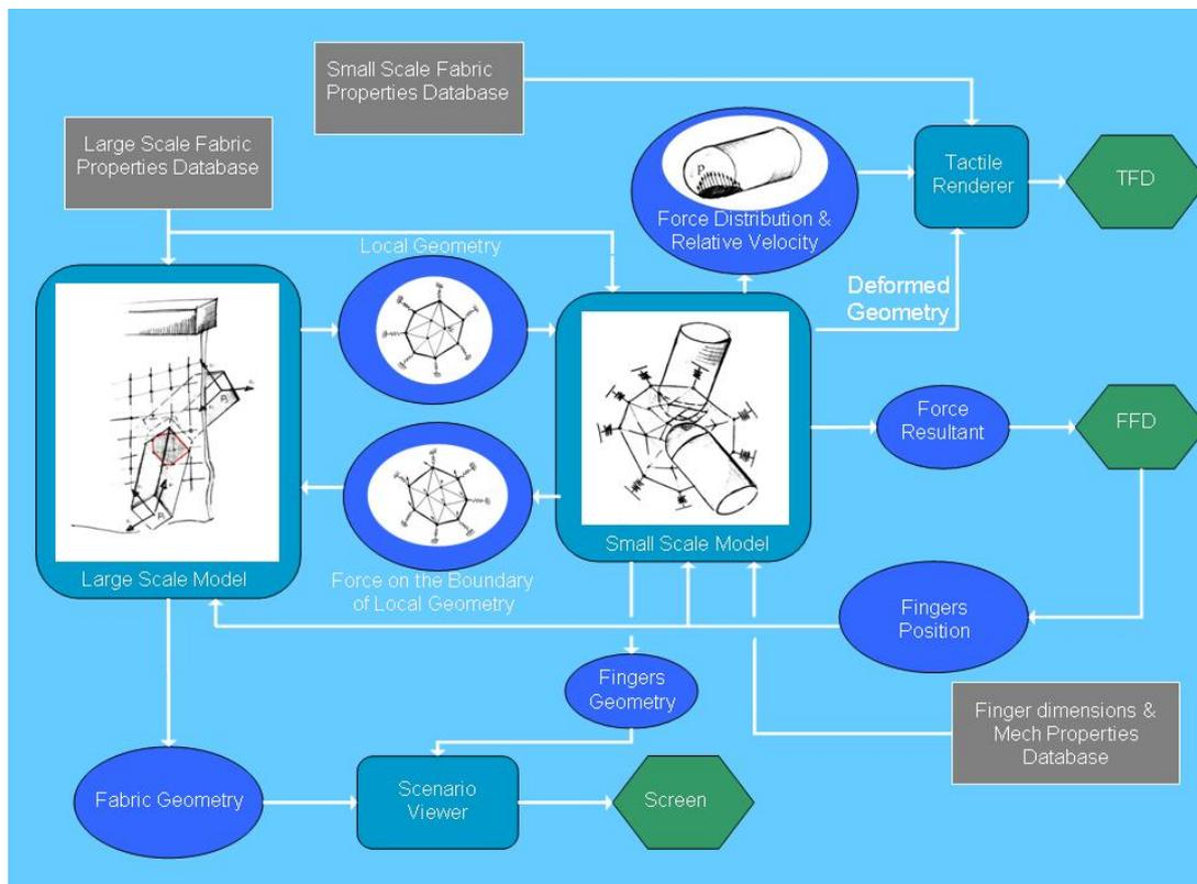
Fig. 2 - Scheme of the architecture of the HAPTEX system.
