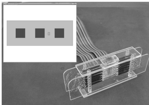
Figure 1. The tactile stimulator. The 24 contactors are central on the upper surface. In the inset screen shot, the tactile cursor which represents the stimulated area is visible between two of the square targets.
