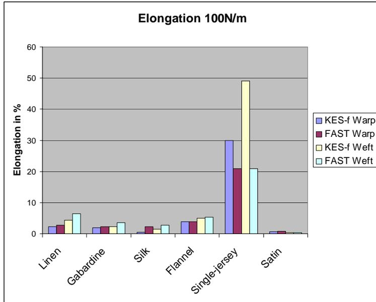
Figure 1: Elongations at 100N/m from KES-f and FAST
