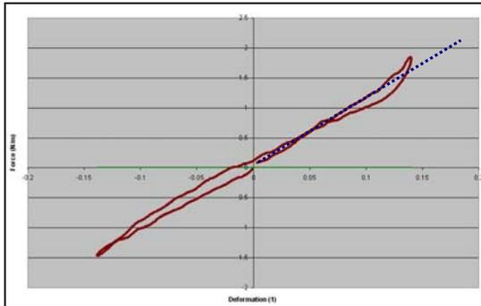
Figure 7: KES-f shear data for silk
