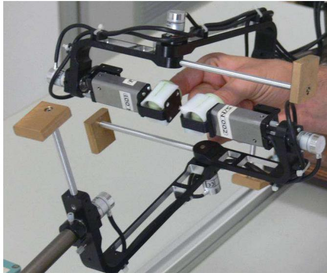
*Figure 3. Two digit interaction with the two GRAB devices, showing the instrumented gimbals and the force sensors which carry the end effectors.*
