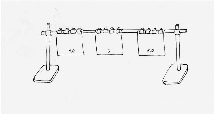
*Figure 3.1 Sample (S) and reference fabrics (1.0, 5.0) holding arrangement (a sketch).*
