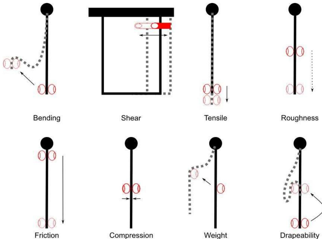
Figure 3.2 Finger positions and manipulation of each property.
