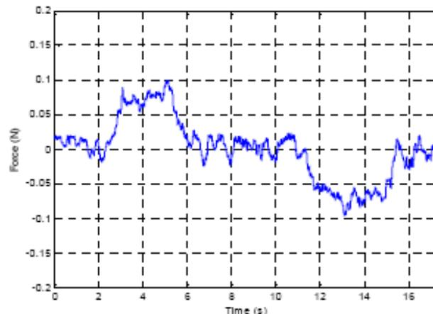
*Figure 4. Force versus time during finger tracking at constant velocity*
