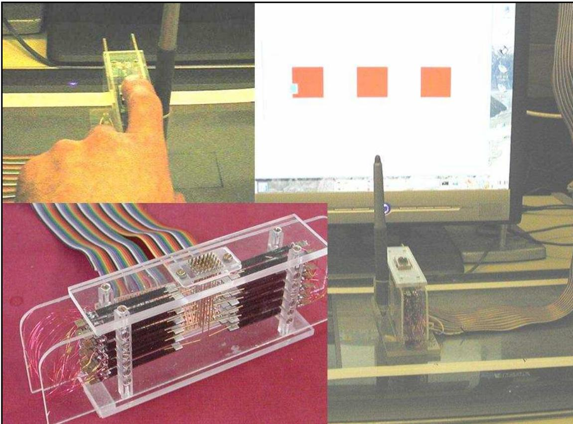
*Figure 5. System for DL2, showing (right) the visual display and the tactile actuator with graphics tablet to provide positional information in 2D; (left) the position of the finger and a view of the tactile actuator.*
