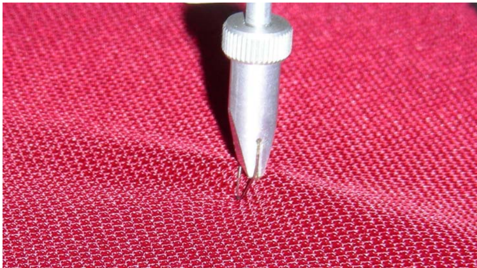
Figure 3.3.4 Fabric stretching and accumulation and yarn twisting during roughness measurement e.g. as a consequence of changing the sensitivity area.
